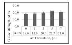
Fig. 4. The tensile strength vs. APTES Silane amount
