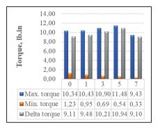
Fig. 2. The torques vs. APTES Silane amount
