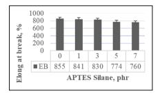
Fig. 3. The elongation at break vs. APTES Silane amount
