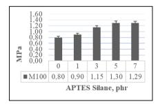
Fig. 5. The modulus at 100% elongation (M 100) vs. APTES Silane amount
