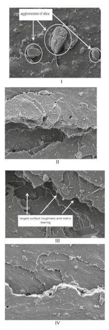
**Fig. 7.** Scanning electron microscopy images of the failed fracture of NR/silica composites with/with no APTES Silane, at a magnification of 500x: (I) No APTES Silane, (II) APTES Silane at 3 phr, (III) APTES Silane at 5 phr, and (IV) APTES Silane at 7 phr.
