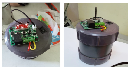
Fig. 3. The design of a simple digital calorimeter
