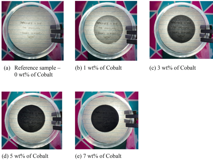
Fig. 1. Digital photograph of the fabricated Co-MRE for (a) reference sample, (b) 1 wt% - Sample 1, (c) 3 wt% - Sample 2, (d) 5 wt% - Sample 3, (e) 7 wt% - Sample 4.
