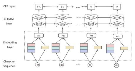
Fig. 2. Overall structure of the model.
