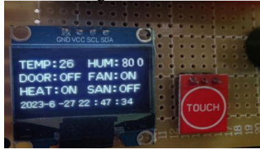
Fig. 11. Activated fan when humidity is greater than 80
