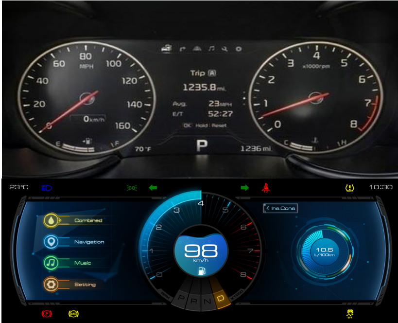
Fig. 1. Mechanical-pointer instrument and full-LCD instrument.
