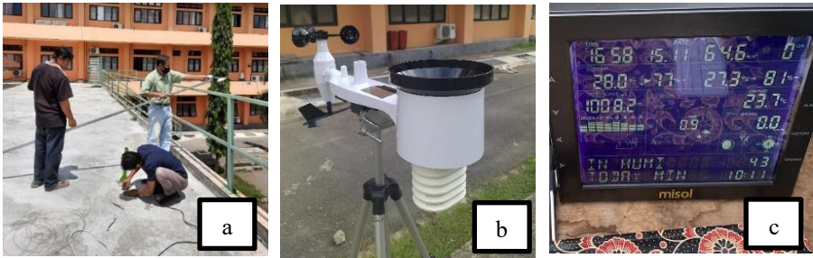
Fig. 2. Installation of AWS for observing climate data outside the greenhouse (a and b) and AWS display devices placed inside the greenhouse (c)
