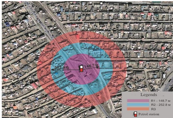
Fig. 7. Explosion boundary zone of a petrol station
