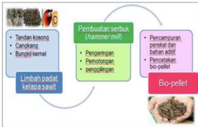
Fig. 6. Figure Flowchart of Bio-pellet Manufacturing Process. Source: Palm Oil Waste Utilization Journal, (Hidayat & Amirta, 2011)
