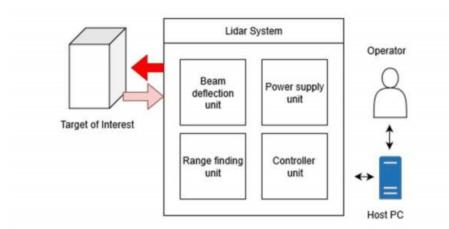
Fig. 3. LiDAR Scanning framework.
