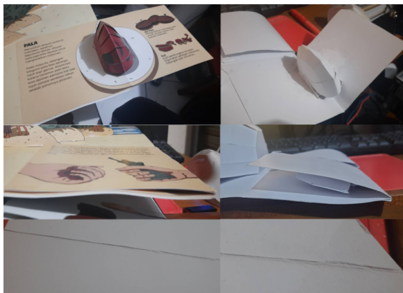
Fig. 5. Comparison between 210 GSM (Left) and 250 GSM (Right). Opened (Top), Closed (Middle), and Spine Wrinkle Comparison (Bottom).
