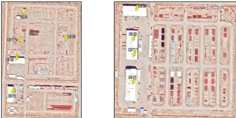
Fig. 8. CPTu and SPT boreholes location in warehouse and drilling storage
