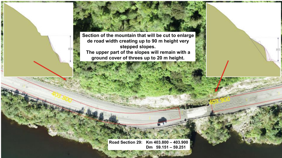
Fig. 5. Possibility of a generalized shear failure of the fractured rock slope, both before the planned blasting works, and after those works, considering the use of presplitting in the blasting plan
