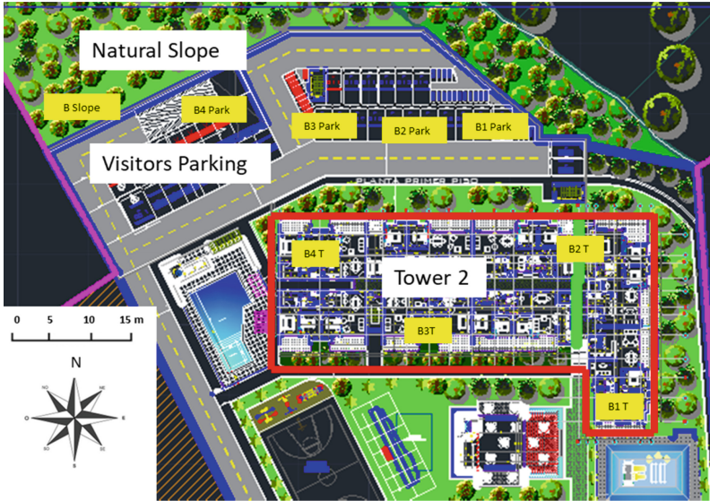
Fig. 1. Masterplan, identifying the location of the tower 2, borings, parking, and natural slope.
