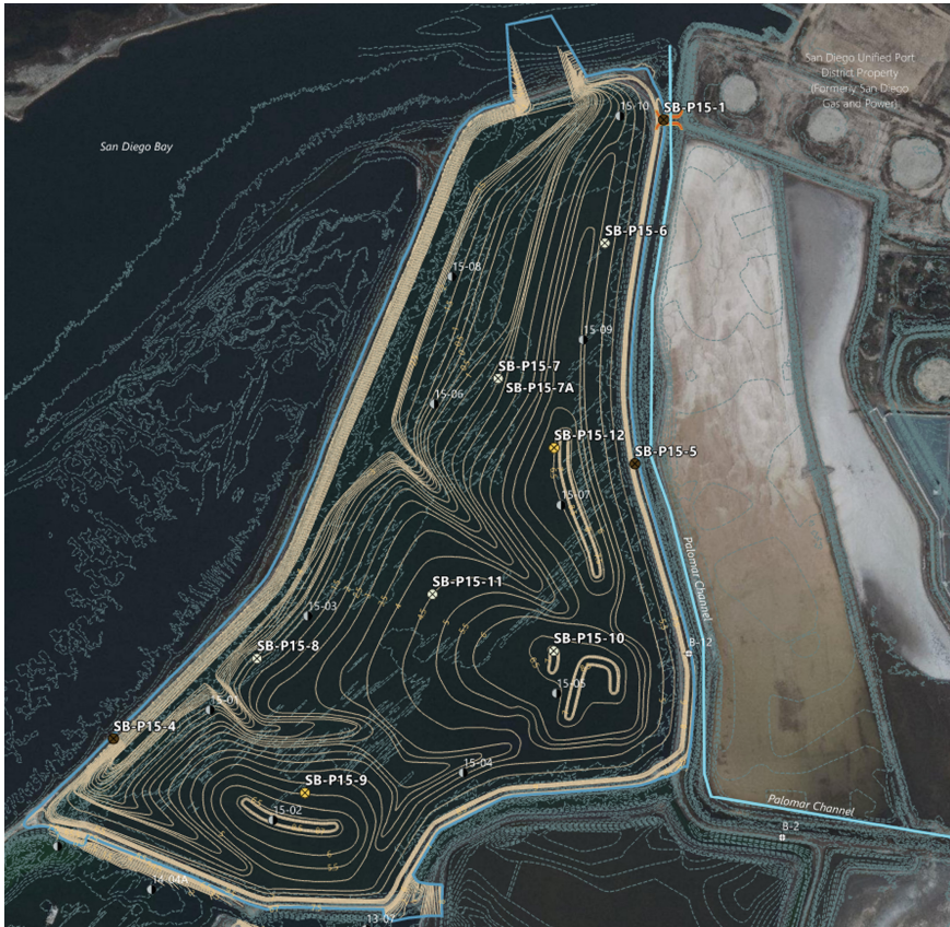
Fig. 2. Subsurface Investigation Map Within Pond 15. Aerial photograph provided by Esri streaming service
