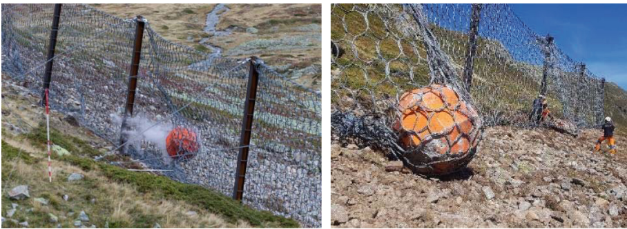
Fig. 5. Example of a random eccentric impact into the instrumented rockfall barrier during a field test campaign
