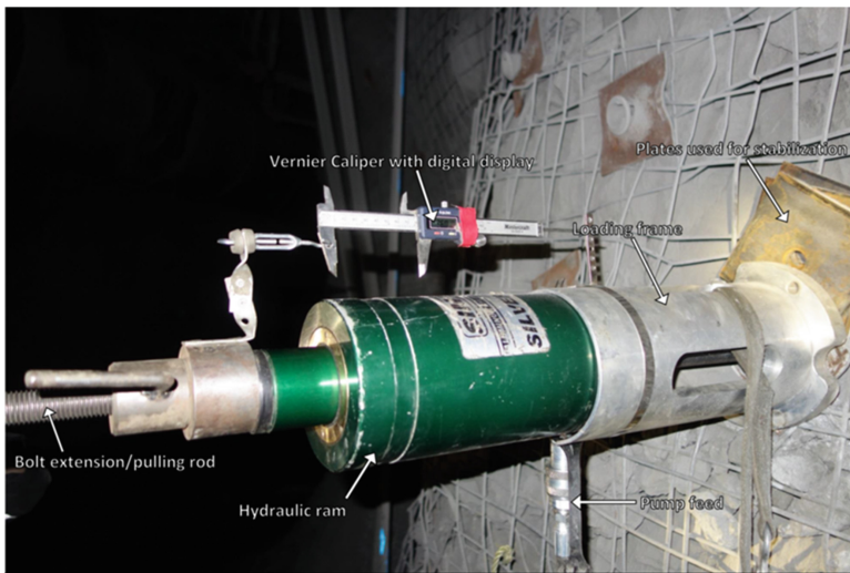
Fig. 4. In situ rockbolt pull test set-up
