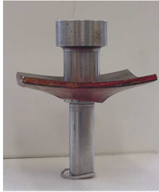
Fig. 3. Steel plate load test
