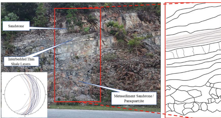
Fig. 4. Typical field sketch of outcrop locality for the rock slope and respective stereographic plots interprets for kinematic analysis planar sliding (dip angle average at 20^\circ \pm 10^\circ )
