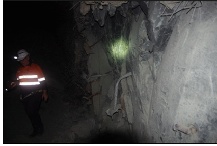
Fig. 2. Anisotropic host rockmass, steep foliation subparallel to N-S oriented walls.
