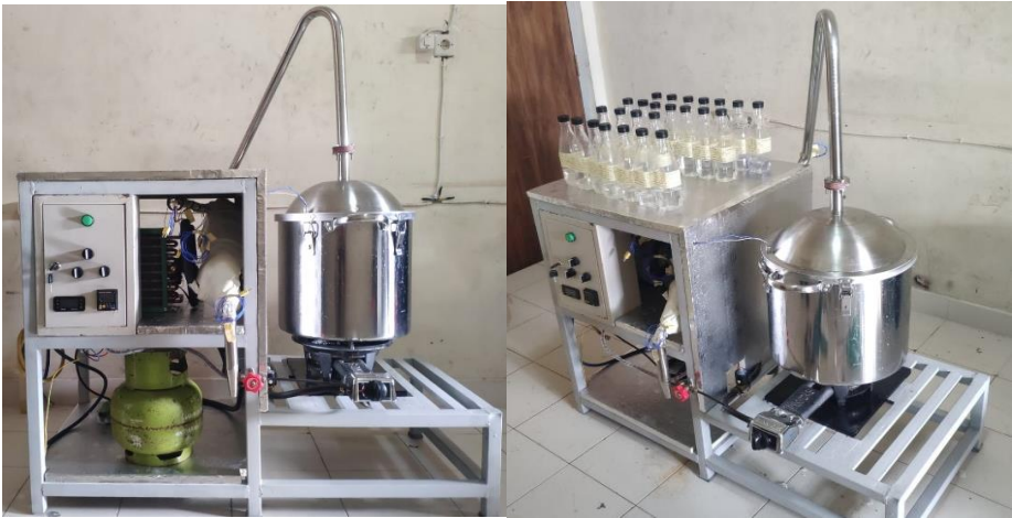
Fig. 1. The established distillation machine completed with refrigerated distiller, smart controller and large boiler tank
