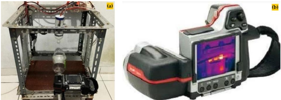
Fig. 2. (a) apparatus setting of freeze-valve study with (b) thermal camera
