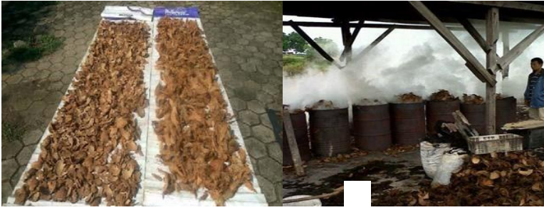
Fig. 1. Specimen production: coconut waste drying process as raw material for briquettes and carbonizing at 6 hours
