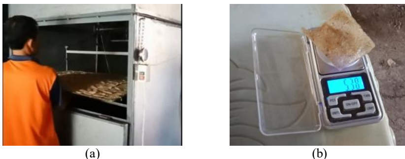
Fig. 2. The process of drying karak rice food uses briquettes as fuel: (a) food drying machine, (b) measurement of the mass of the drying product
