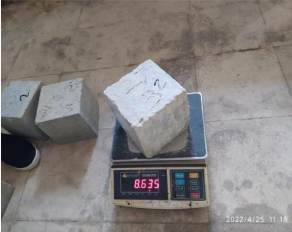
Fig. 2. Concrete compressive strength test object in the shape of a cube
