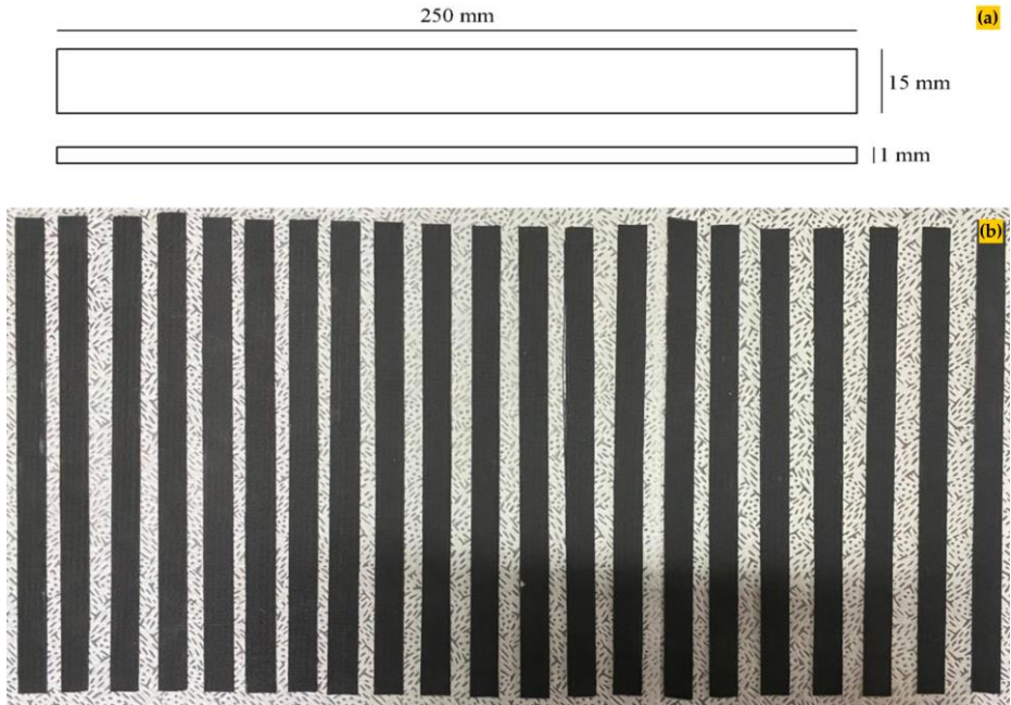
Fig. 2. The detail of (a) ASTM D3039, and (b) sample after cut
