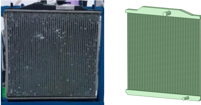
Fig. 2. Radiator domain 3D model
