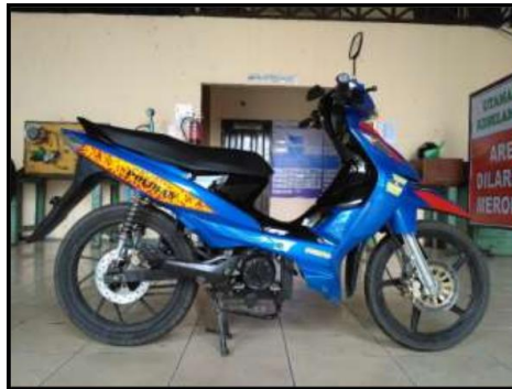
Fig. 1. Conversion of Suzuki SP125 Electric Vehicle (EV)
