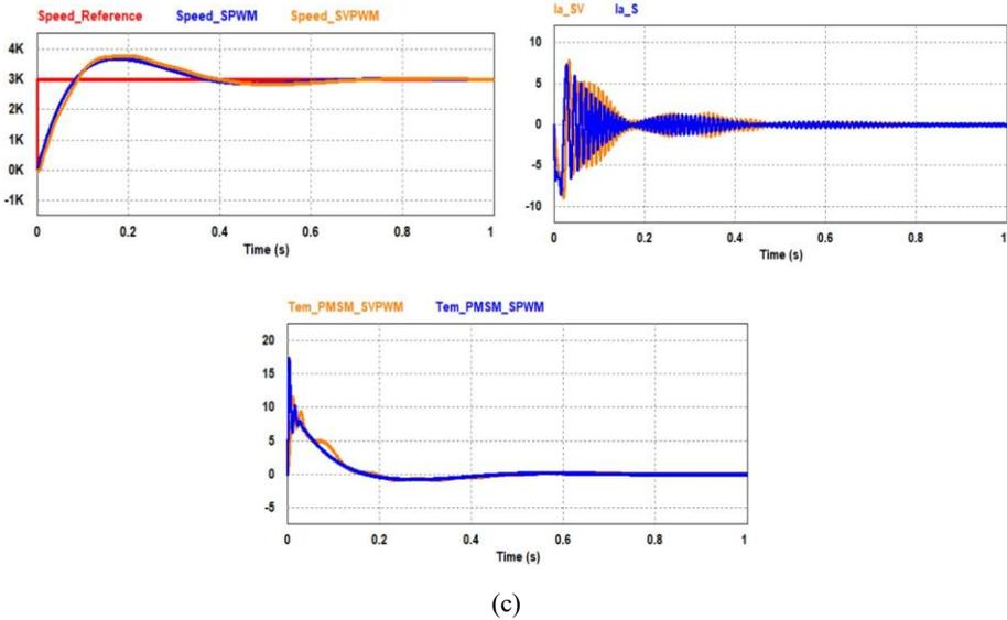
**Fig. 3.** Permanent Magnet Synchronous Motor (PMSM) Performance at Constant Speed 3000 RPM No Load. (a) Speed Response (b) Current (c) Torque
