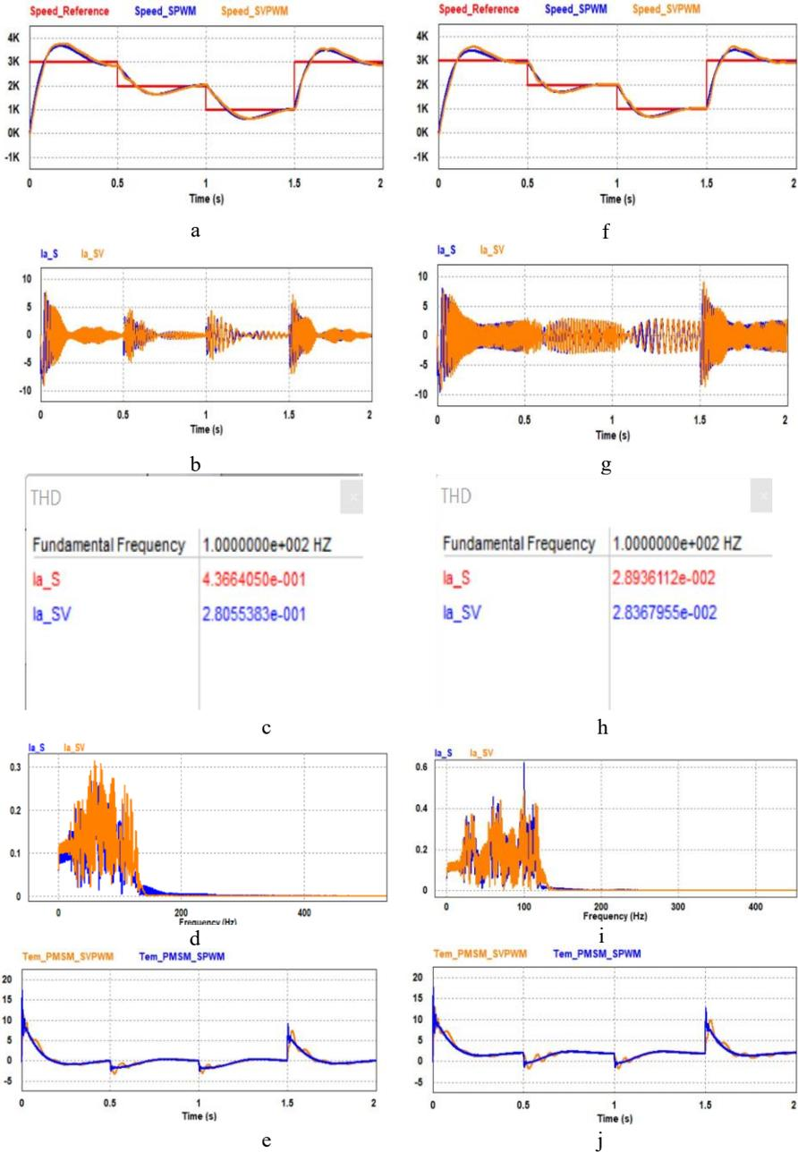
**Fig. 5.** PMSM Performance at Dynamic Speed No Load and With Load. (a) Speed Response No Load (b) Current No Load (c) THD No Load (d) Current Spectrum No Load (e) Torque Ripple No Load (f) Speed Response 2 Nm Load (g) Current 2 Nm Load (h) THD 2 Nm Load (i) Current Spectrum 2 Nm Load (j) Torque Ripple 2 Nm Load
