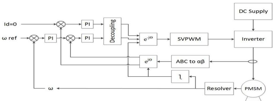
**Fig. 1.** Field Oriented Permanent Magnet Synchronous Motor (PMSM) Control Diagram Block
