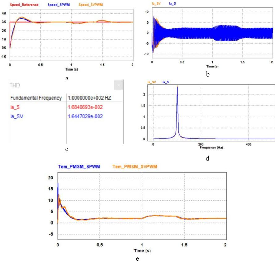
**Fig. 6.** PMSM Performance at Constant Speed With Load Disturbance. (a) Speed Response (b) Current (c) THD (d) Current Spectrum (e) Torque Ripple
