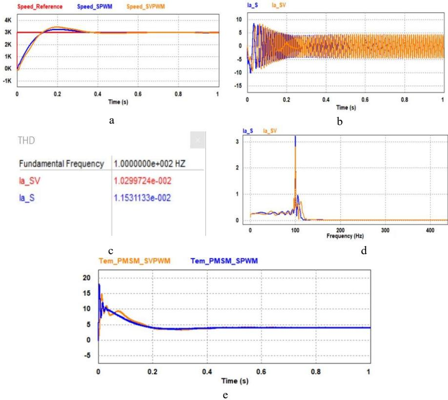
**Fig. 4.** PMSM Performance at Constant Speed 3000 RPM With 4 Nm Load. (a) Speed Response (b) Current (c) THD (d) Current Spectrum (e) Torque Ripple
