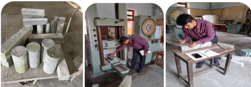
Fig. 4. Testing of Cubes, Cylinders, Prisms for its Mechanical Properties
