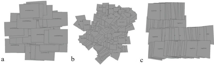
Fig. 1. Different types of flight (a) manual (b) semi-autonomous (c) autonomous, Nex et al. 2014 [3].
