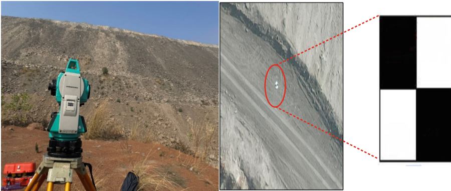
Fig. 3. Total station for GCPs acquisition and photogrammetric targets for GCPs.
