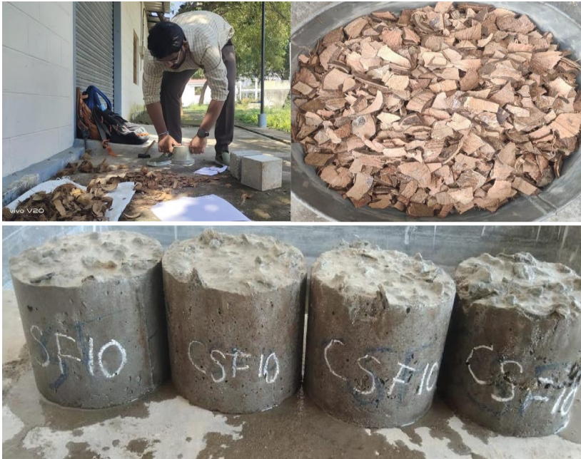
Fig. 1. Showing the crushing technique, crushed Coconut Shells and Cantabro specimens
