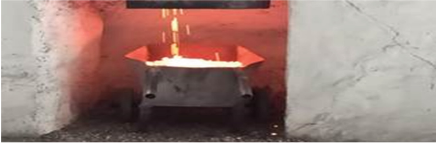
Fig. 4. Nodules not being dispensed properly into the trolley.
