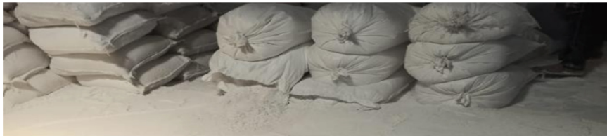
Fig. 2. Raw-Mix bags burst due to excess pressure.
