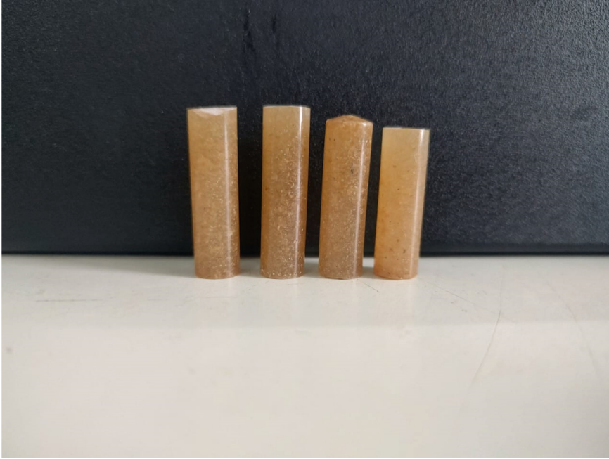
Fig. 1. Chitosan epoxy polymer composites Pin on Disc test specimen
