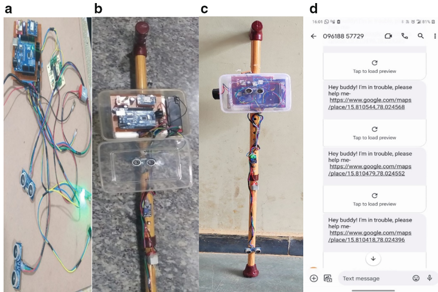
Fig. 2. The proposed blind stick results a) Blind stick initial circuit b) Internal structure of blind stick c) Complete structure of sophisticated smart blind stick d) Message to the guardians when he/she's in danger
