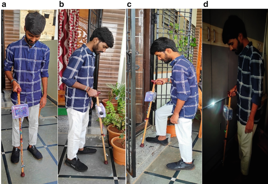
Fig. 3. a) Person holding it b) Stick detecting the obstacle and ringing the buzzer c) Stick helping the person on stairs d) LDR turning on in the absence of light
