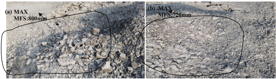
Fig. 14 Photograph of fragmentation with S/B ratio 1.2 & S/B ratio 1.3
