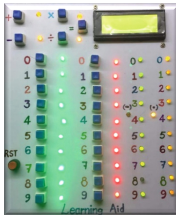
Fig. 8. Prototype of Ganitha Sahaya – Math tool for special education.
