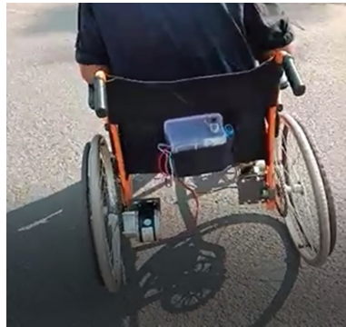
Fig. 10. Control Circuit board in a pocket stitched at the backrest of wheelchair
