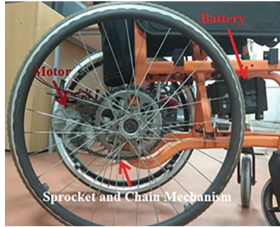
Fig. 1. Sprocket and Chain Mechanism
