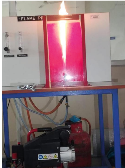
Fig. 4. Test rig for flame propagation of R1234yf/R134a
