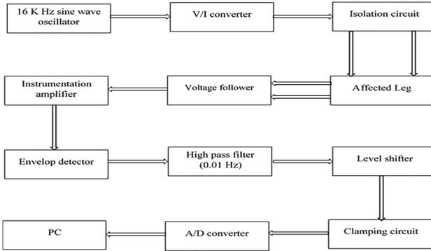
**Fig. 1.** Basic components of the IPG system.
