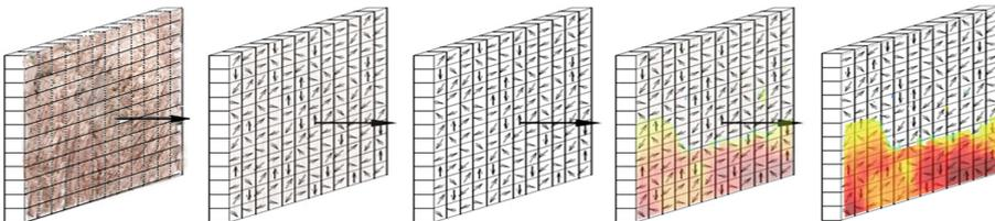
**Fig. 4:** 2D deformation images of the wall generating deformation heatmaps (Source: Ground-Probe SSR)
