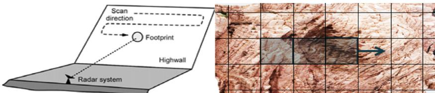
**Fig. 2:** Slope Stability Radar (SSR) scanning pattern (Source: GroundProbe SSR)
