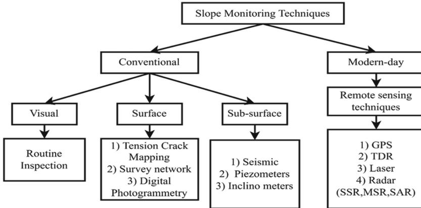
**Fig. 1:** Classification of slope monitoring techniques
