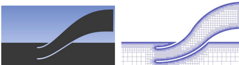
Fig. 4. Cross-sectional view of the Computational Domain (Left) and the Mesh (Right)
