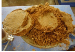
Fig. 11. Rupture of geotextile discs in case of soil samples modified with 5% cement content
