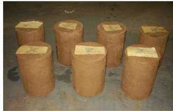
Fig. 4. Prepared cylindrical soil specimens of desired density for UCS testing.
