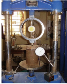
Fig. 2. Unconfined compressive strength test set up
