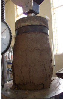
Fig. 7. Bulging failure pattern of reinforced plain murrum soil sample
