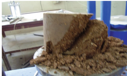
Fig. 6. Shear failure pattern in case of failed samples of plain murrum soil
