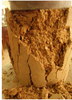
Fig. 8. Splitting failure in case of 2% cement modified murrum sample
