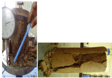
Fig. 5. Shear failure pattern in case of failed samples of plain murrum soil
