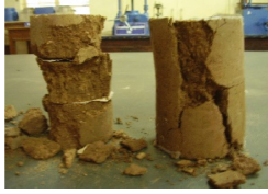
Fig. 9. Failed murrum soil samples with 2 layers of geotextile (Fibertex G-100 and PD 381)
