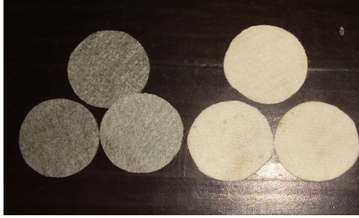
Fig. 1. Fibertex G – 100 and PD 381 geotextile cut into circular discs used for the study
