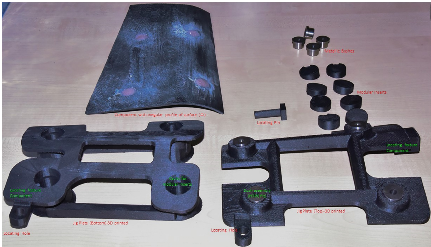
Fig.3. 3D printed parts of a jig assembly
