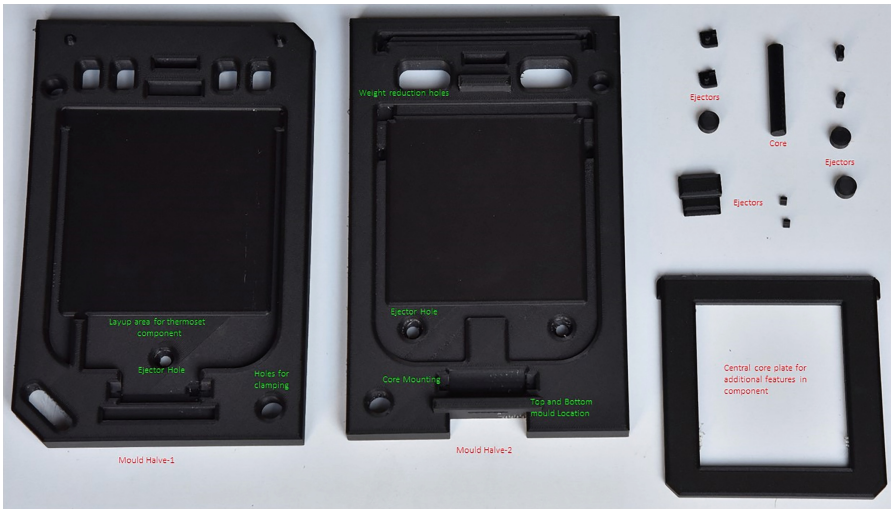
Fig.2. 3D printed Matched-Die Mould
