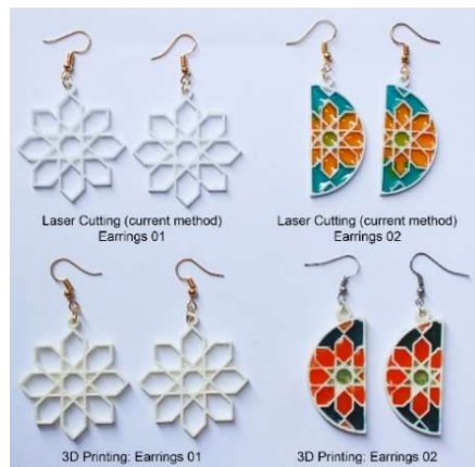
Fig. 5: The final prototypes made for the case study through the current methods and the 3D printing method.
