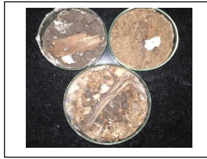
Figure 3 Petri plates with wood samples covered with soil, a substrate, and 5% Cellulose powder.
