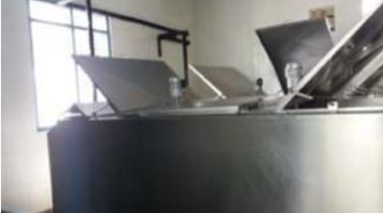
Fig. 1. The Packo milk cooling system, provided by KUD SAE Pujon.
