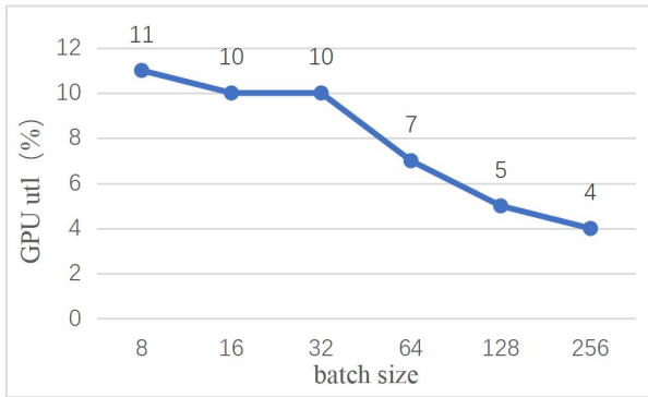
Fig. 1. The trend of GPU utilization under different batch sizes (Photo/Picture credit: Original).
