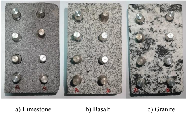
Fig. 3. Preparation of drawing specimen.
