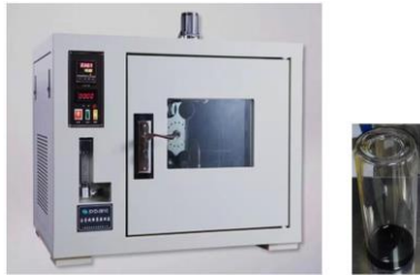
Fig. 1. Rotating film oven and aging bottle.
