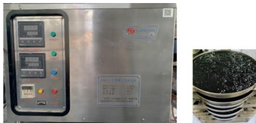
Fig. 2. PAV aging test chamber and asphalt sample after PAV aging.
