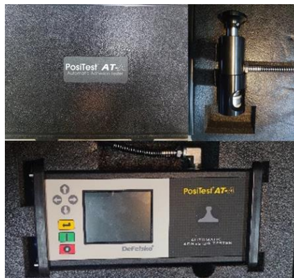
Fig. 4. Posi Test AT-A automatic digital display puller.
