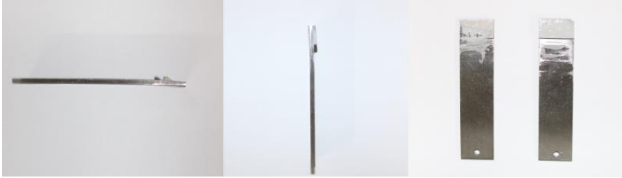
Fig. 6. Failure occurred within the adhesive layer
