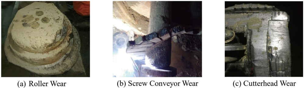
Fig. 1. Shield Tunneling Equipment Wear Diagram
