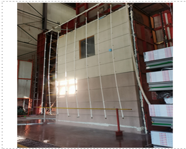
Fig. 7. Performance evaluation of the self-insulation wall system with two layers of different dry density of AAC
